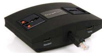
Cable chamber with optional Ethernet cable.
